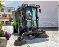
As standard the hopper has a rotation filter system and a fresh water tank with 190 I capacity.
