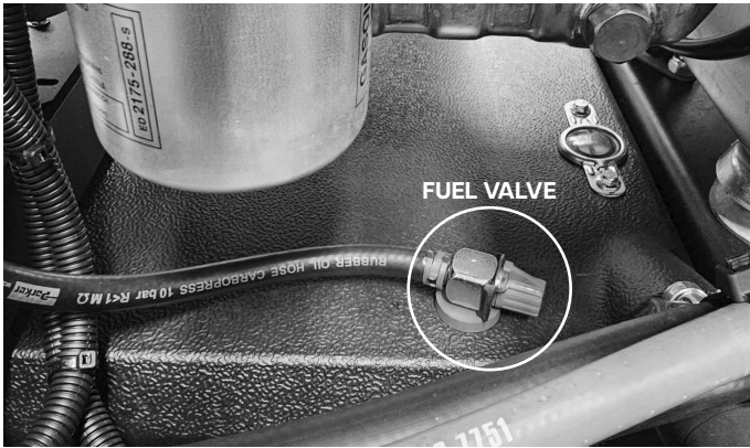
Figure.8 - Fuel Valve Location
