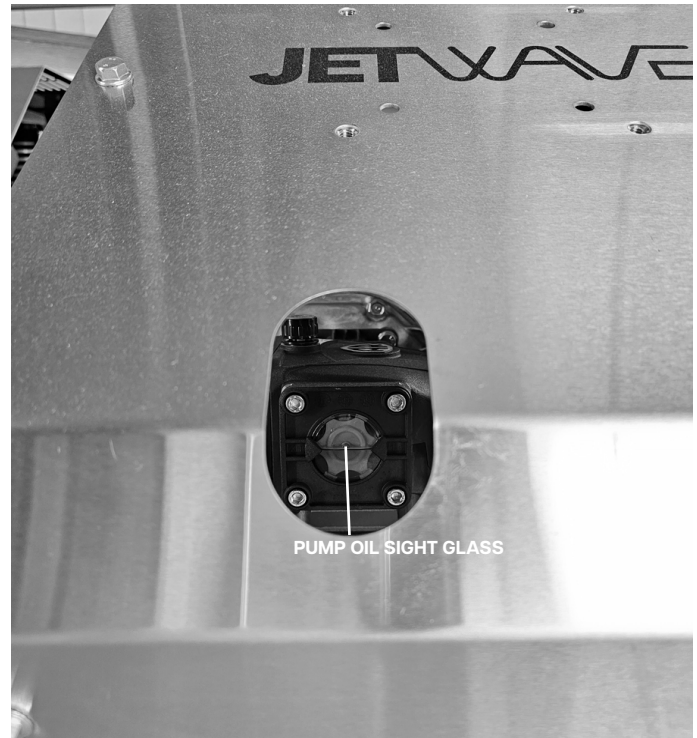
Figure.8 - Checking Pump Oil Level
