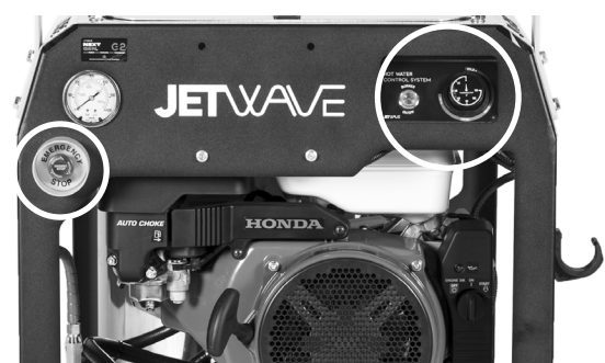
Figure.8 - Explorer G2 E-Stop & Burner Operation
