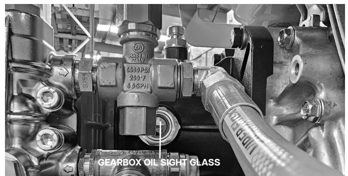
Figure.11 - Checking Pump and Gearbox Oil Level
