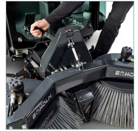
Change of attachments - no tools required.
